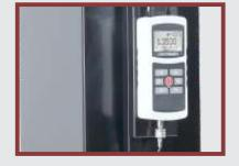
Single column tabletop system for force testing
