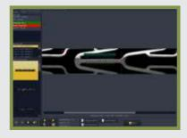
Measures horizontal, vertical, angular dimensions and linear-radial symmetry
